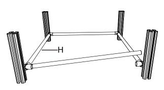
Insert the Round Rail into the 90° Rail Connector to connect the 4 sets of 76 x 76mm Posts.
