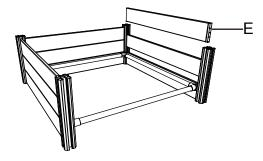
Use the 152 x 22mm Panel - L to assemble the three side panels of the Whelping Box.
