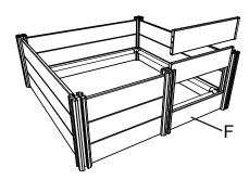
Use the 152 x 22mm Panel - S and 76 x 76mm Post to assemble the front door of the Whelping Box.
