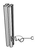
Place the 90  $^\circ\,$  Rail Connector on the Rail Connector Clamp.
