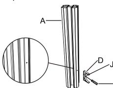
According to the reserved hole on the 76 x 76mm Post, screw the Rail Connector Clamp on the 76 x 76mm Post.
